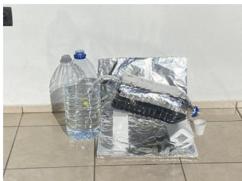
Prototype of the solar desalination system
